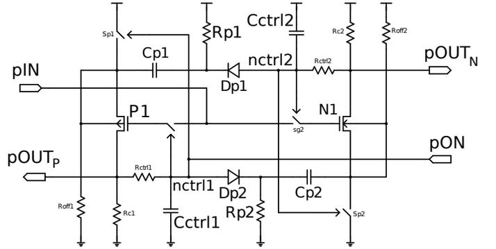
Fig. 7. A simplistic embedded redundancy circuit. This circuit is symmetric except for the different ageing effects in  $N1$  and  $P1$ .
