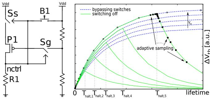
Fig. 4. The Halting Problem. The voltage at  $nctrl$  controls the switches  $Sg$  and  $Ss$ .  $|\Delta V_{th}|$  in  $P1$  varies over time, and causes a shutdown. Circles mark the computed second-time steps, those at filled circles are introduced by the shutdown.
