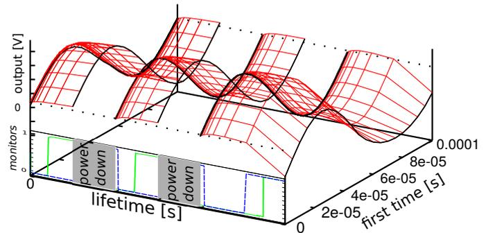
Fig. 6. Monitoring the power stage: The failure signals (front) indicate too high (green) and too low (blue, dashed) offset peaks.
